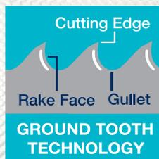
Teeth are ground to very fine tolerances which achieve significantly higher cutting efficiency than standard blades
