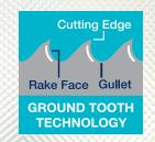
Teeth are ground to very fine tolerances which achieve significantly higher cutting efficiency than standard blades BRANDS
