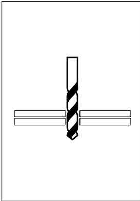
Drill hole through materials to be riveted.
