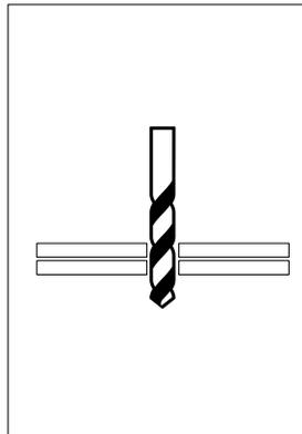
Drill hole through materials to be riveted.
