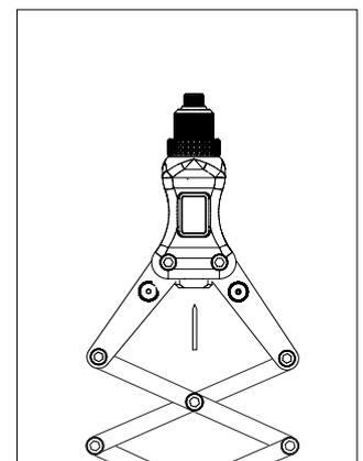
Open lattice fully to remove rivet stem.
