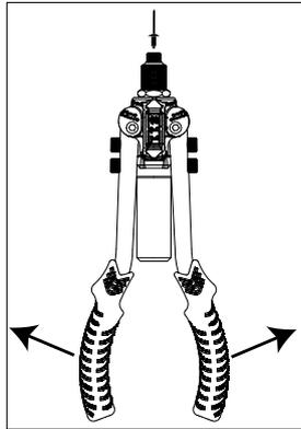
Open handles to insert rivet.
