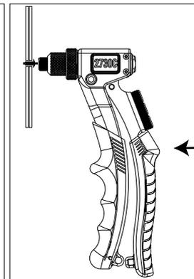
Squeeze handle to fix rivet. Repeat until rivet snaps.
