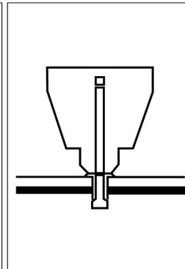
Insert the riveter into the hole.
