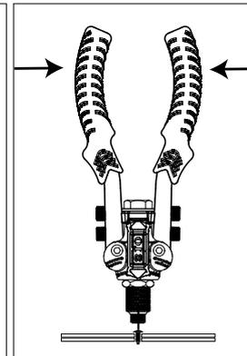
Close handles to fix rivet. Repeat until rivet snaps.
