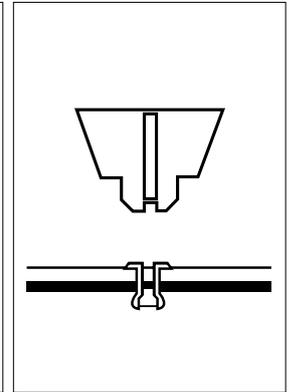
Remove riveter and open handles fully to remove rivet stem.
