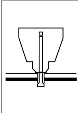
Insert the riveter into the hole.
