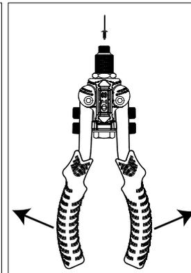
Open handles to insert rivet.
