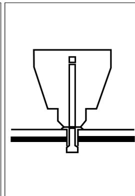
Insert the riveter into the hole.
