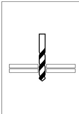
Drill hole through materials to be riveted.
