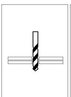
Drill hole through materials to be riveted.
