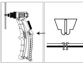
Squeeze handle to fix rivet. Repeat until rivet snaps.
