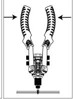
Close handles to fix rivet. Repeat until rivet snaps.
