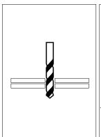
Drill hole through materials to be riveted.
