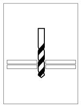
Drill hole through materials to be riveted.
