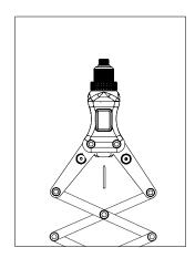
Open lattice fully to remove rivet stem
