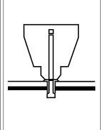
Insert the riveter into the hole.
