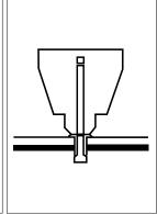
Insert the riveter into the hole.
