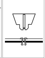
Remove riveter and open handles fully to remove rivet stem.
