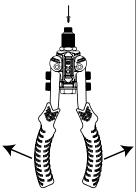
Open handles to insert rivet.
