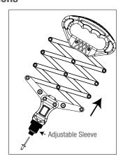
Extend Lazy Tong Riveter, insert rivet and adjust sleeve if required.
