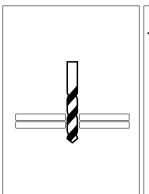
Drill hole through materials to be riveted.
