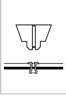
Remove riveter and open handles fully to remove rivet stem.
