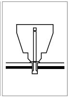
Insert the riveter into the hole.
