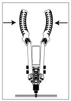
Close handles to fix rivet. Repeat until rivet snaps. The rivet stem falls into the collector.
