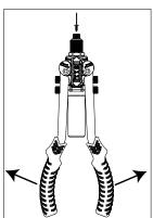
Open handles to insert rivet.
